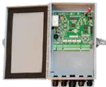
Inside of FlexZone processor
