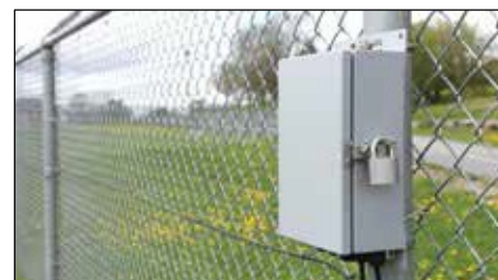
FlexZone processor on a fence
